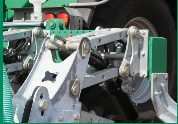
The parallelogram hitch ensures precise depth control for each row. This means the slurry is always placed at the preset height.
