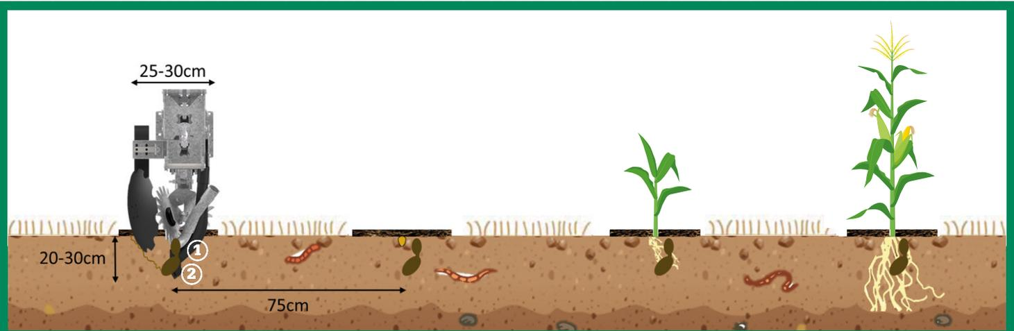
SAMSON Strip-Till workflow is functional and extremely precise. The slurry is placed in two lines: ① approx. 30 % in the upper and ② approx. 70 % in the lower slurry line.
