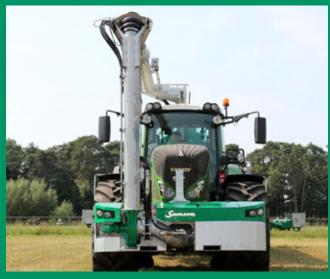
Side-mounted filling arm ensures optimal visibility from the cab.
