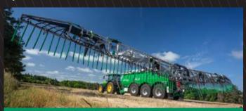
Two ultrasonic sensors continuously measure the height from the frame of the SHB4 drip hose boom to the soil surface. At the same time, the side wings of the SHB4 boom are controlled independently of each other both above and below level. This ensures that the hoses are always in contact with the soil surface and that the slurry is applied in narrow strips with the least possible surface area and thus the least possible volatilisation of ammonia, even on rough terrain.
