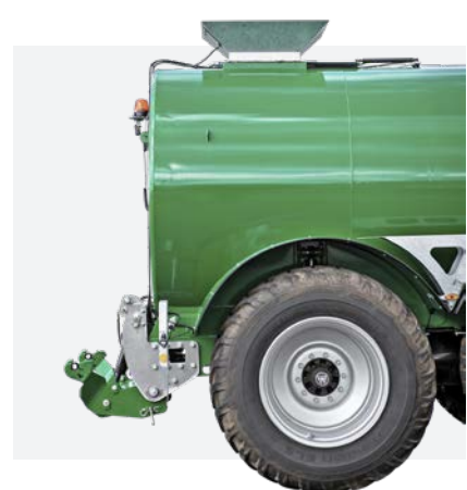
External filling Wide filling funnel with removable valve plate, venting valve and safety valve. The funnel can be opened via a hydraulic slide valve to allow external filling from a stationary or mobile pump unit.
